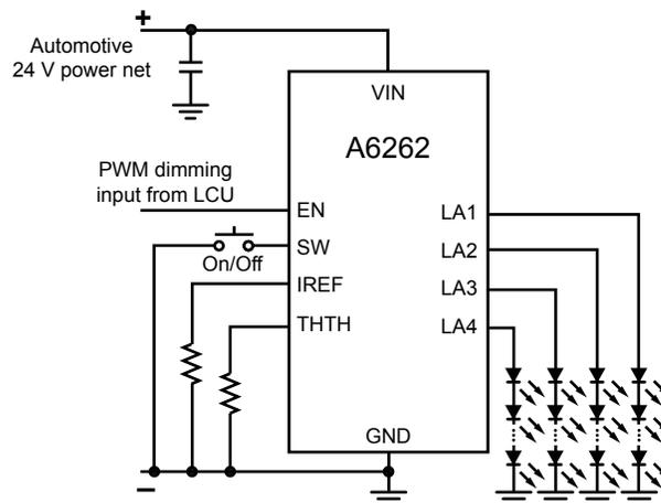
Figure 10. Typical applications using SW and EN together.
